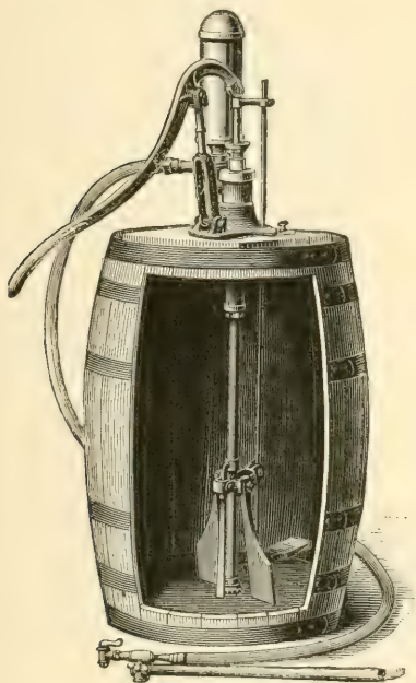
FIG. 33.—An undesirable type of barrel sprayer—now off the market; the air-chamber and other parts above the barrel render it top-heavy, and may be easily broken.
